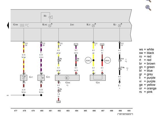
Oil pressure switch, Ambient temperature sensor, Windscreen washer fluid level sender, Front left brake pad wear sender, Oil level and oil temperature sender, Control unit in dash panel insert
