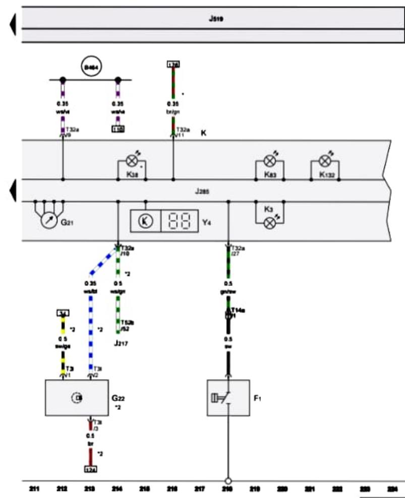
**Oil pressure switch, Speedometer, Speedometer sender,
