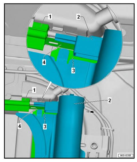
Unscrew bolts of sun blind housing -2- (3.5 Nm).
