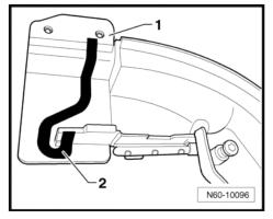
Push entire rear part -1- with discharge tubes -2- in direction of -arrow- onto guide rail -3-.
