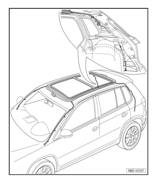
The rear water drain hoses run through the D-pillars and end in the rear wheel housings. Cleaning is done from the wheel housing. The wheel housing liner must be removed.
