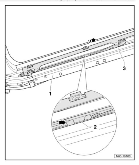
Push glass panel tilting mechanism only on areas -arrow- of slider -2-, not on guide plate -3-.
