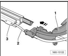
Tighten bolts -3- of rear part -2- on guide rail -1- to 2 Nm.
