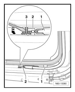
Using a screwdriver, unclip mounting bracket -2- and wind de-
