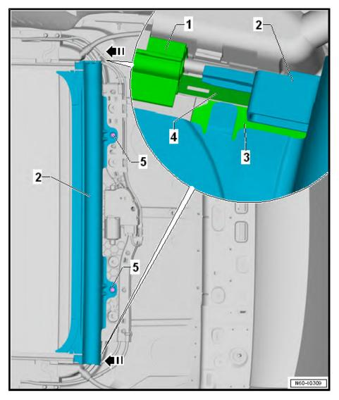
Push sun blind housing -2- parallel with sun blind steel strap -4- in -direction of arrow- into sun blind rail -1-.
