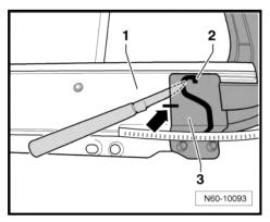
Pull entire rear part -1- with discharge tubes -2- in direction of -arrow- out of guide rail -3-.
