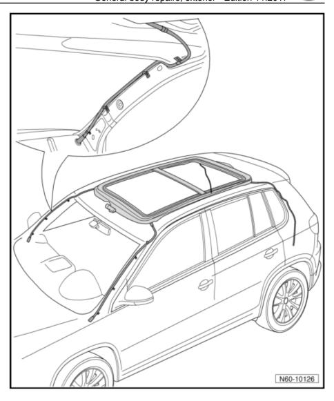
The front water drain hoses are routed in the A-pillars and end in the plenum chamber. Cleaning is done from panorama sliding roof cut-out.
