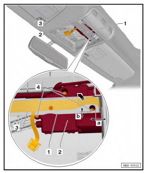
Carefully detach ribbon cable -3- (if fitted) from web -1- and pull it to side -arrow-.
