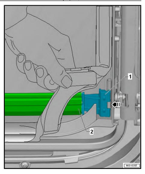
Push sun blind slide -1- in direction of -arrow- into sun blind cross strut -2-.
